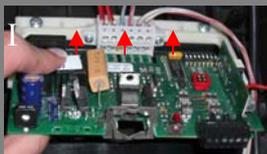
9. Put PCB back in operator (picture I)
