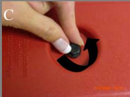
3. Remove the housing (picture C)
