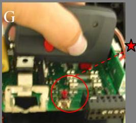
7. Press the preferred button (2 LEDs light up) and hold it till the LED on the PCB turns off (picture G)
